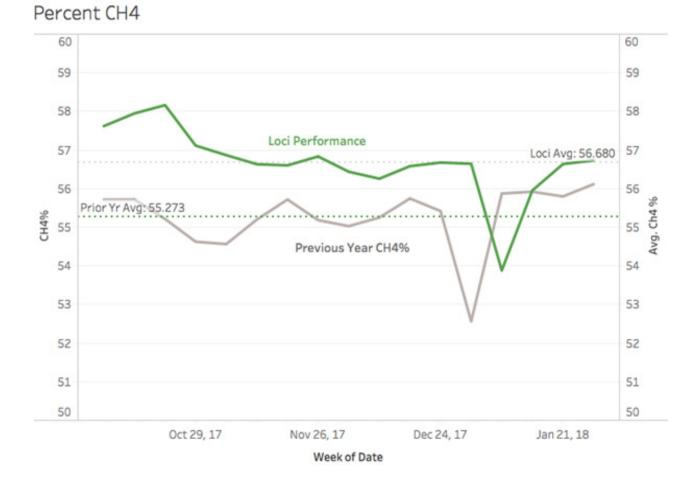
**Figure 3:** Weekly average percent methane composition figures since optimization by Loci started, showing a 1.3% improvement.
