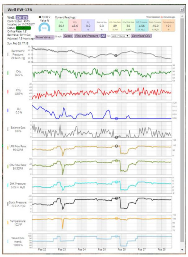
**Photo 3:** WellWatcher<sup>®</sup> user interface, with field level gas collection data. Green icons indicate collection wells that are operating within Aria Energy gas composition requirements, yellow icons indicate wells that are trending towards limits of gas composition.
